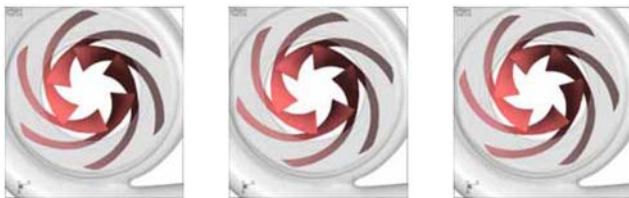
Figure 8 : Three impeller positions for the frozen rotor model
