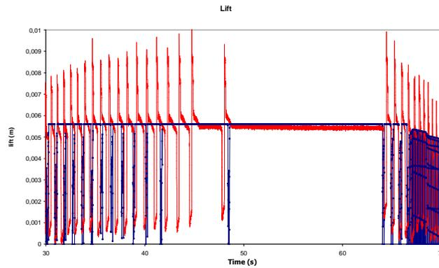
**Fig.14:** Comparison of experimental and calculated lift for 1/2G2 valve
