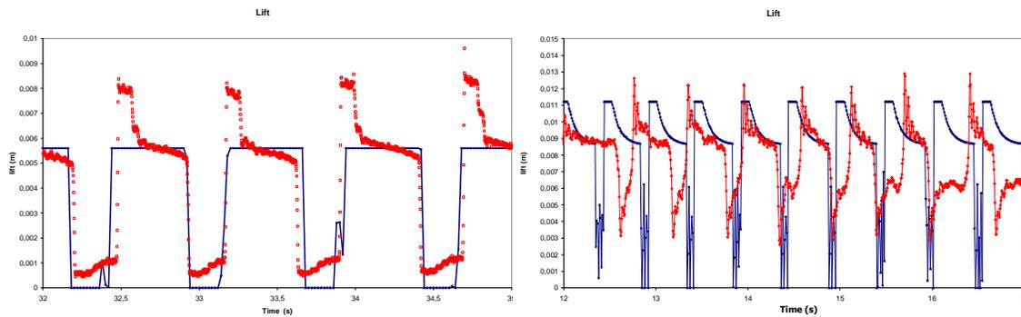
**Fig.15:** Test and simulation of lift during a safety valve test with backpressure for 1/2G3 and 2J3 type safety valves
