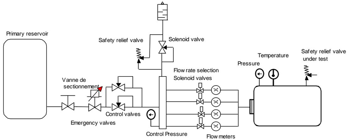
**Fig.4:** CETIM's safety valve test facilities in air
