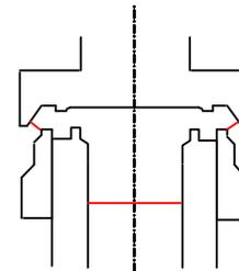
**Fig.12:** The critical pressures ration occurs both in the nozzle and in the lateral area between the nozzle and the disc -
