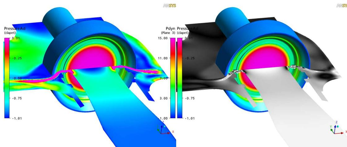
**Fig. 9 :** Dynamic pressure and density gradient; case P1
