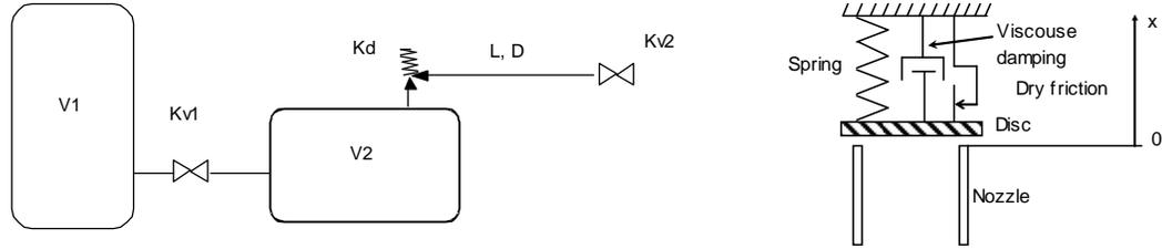
**Fig.10:** Simplified test rig and simple valve model
