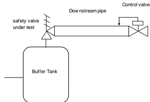
**Fig. 5:** Safety valve under test and back pressure generating system
