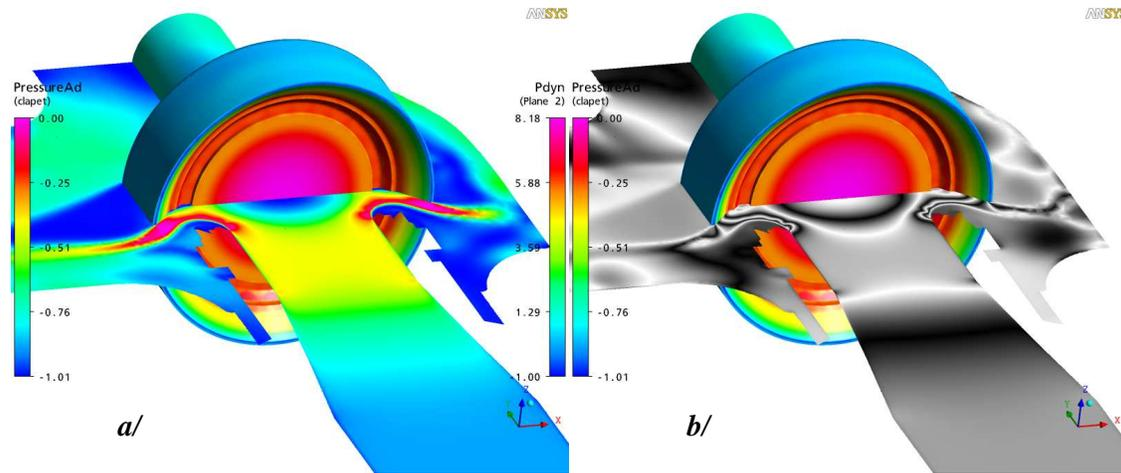
**Fig. 8:** a/ Dynamic pressure acting on disc valve b/ density gradient on x-y plane; case P3
