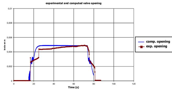
**Fig.13:** Variation of the lift during a safety valve test
