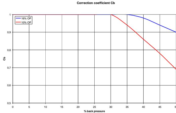
**Fig.2:** Correction coefficient  $C_b$  for compressible flows
