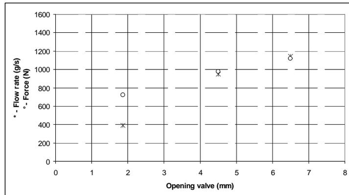
**Fig. 7:** Flow rate and force acting on the valve following the valve opening
