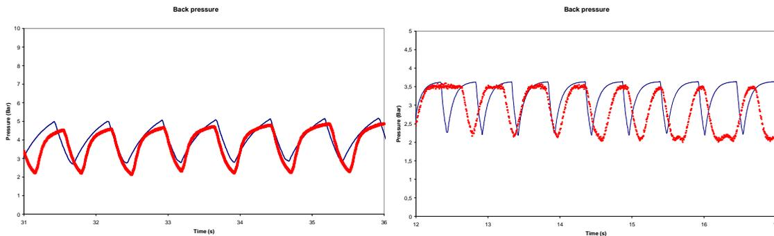
**Fig.16:** Test and simulation of back pressure during a safety valve with backpressure for 1/2G3 and 2J3 type safety valves
