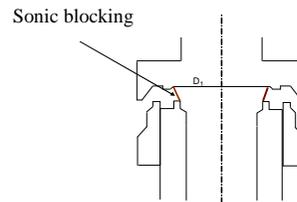
**Fig.11:** The critical pressures ration occurs in the lateral area between the nozzle and the disc - "curtain area"
