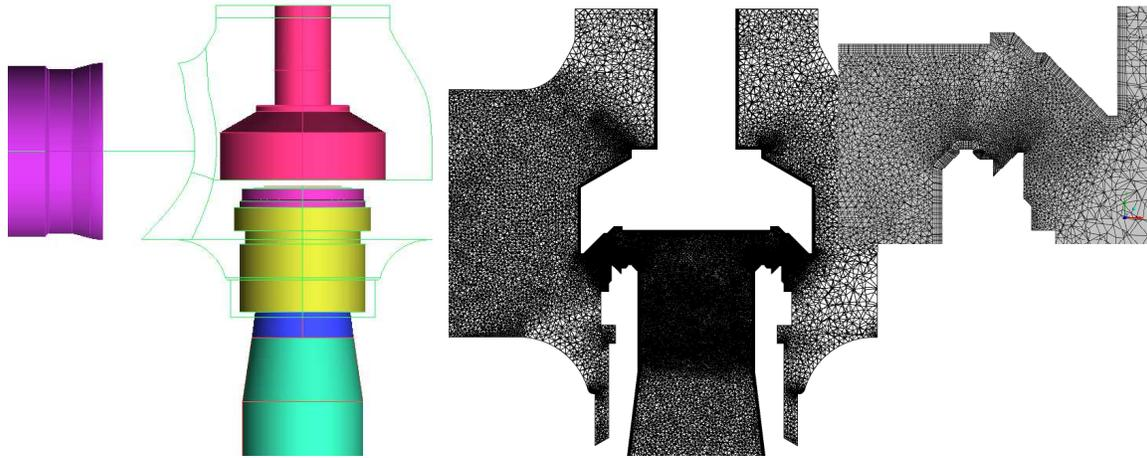
**Fig. 6:** Grid view of the computational domain
