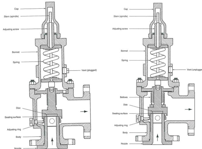
**Fig.1:** Conventional and balanced bellows pressure relief valves [1]
