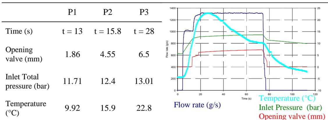
**Tab. 1:** Specifications of three computations corresponding to the different valve openings: data extracted from experimental investigations
