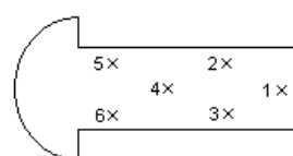
Figure 2. Hardness indentation points distribution on the section
