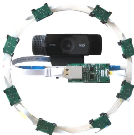
Figure 50 Antenne MEMS 8 microphones
