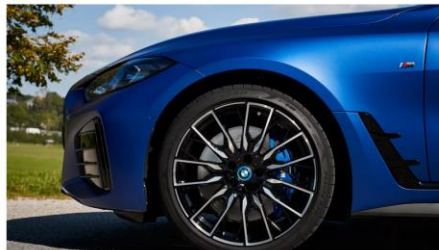
The matt clearcoat of the new BMW i4 M50 in Frozen Portimao Blue was produced without fossil raw materials and is based on organic waste. (Photo: BMW Group)
