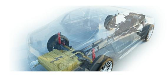
Mechanical, hybrid and electric powertrains: high speed/high power tests, thermal system tests and development of hydrogen tanks
