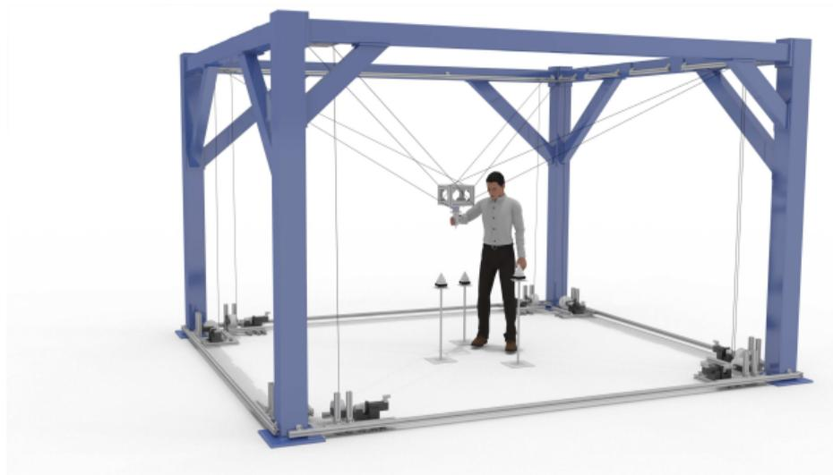
Figure 16: Second Use Case - (UC2) - Co-manipulation of a platform with eight cables
