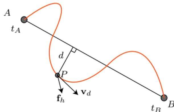
Figure 18: Ideal path (black), end-effector tip path during user experiment (orange)
