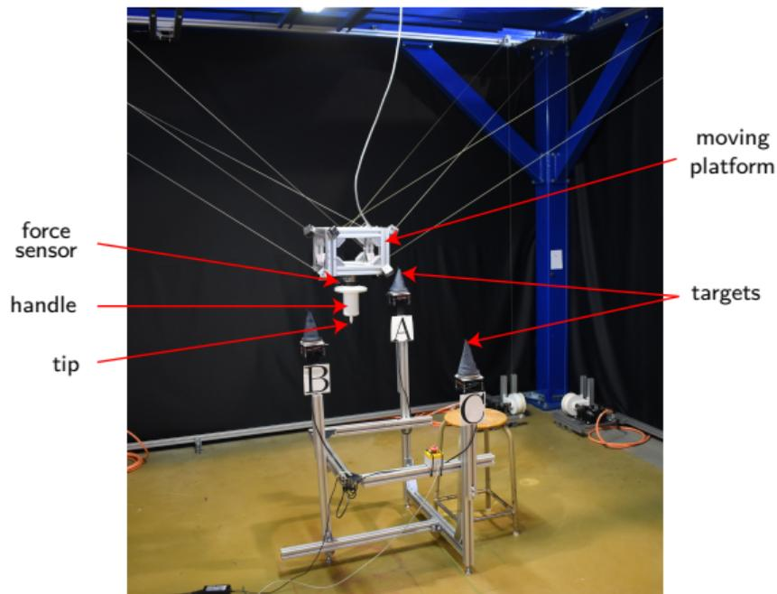
Figure 17: User experiment setup
