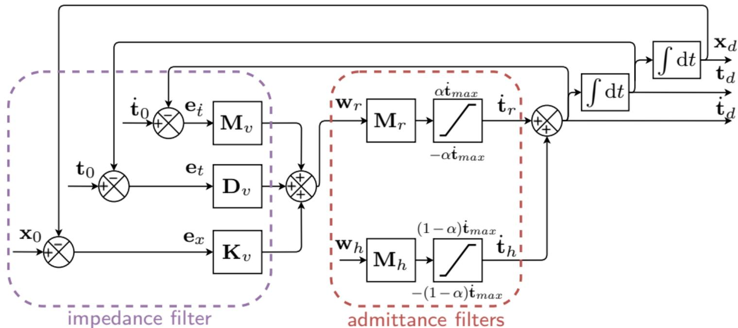
Figure 9: Hybrid control scheme for co-manipulation with a CDPR
