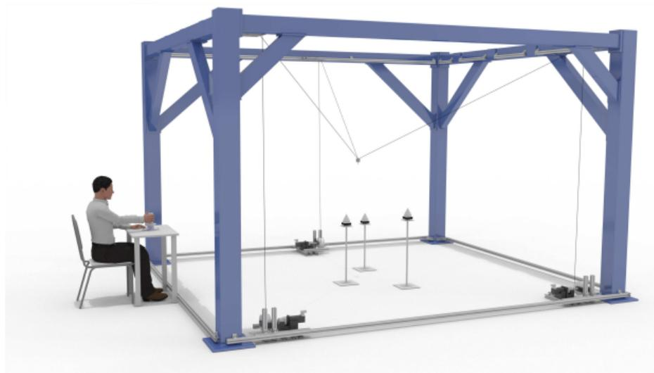
Figure 14: First Use Case (UC1) - Teleoperation of a platform with three cables
