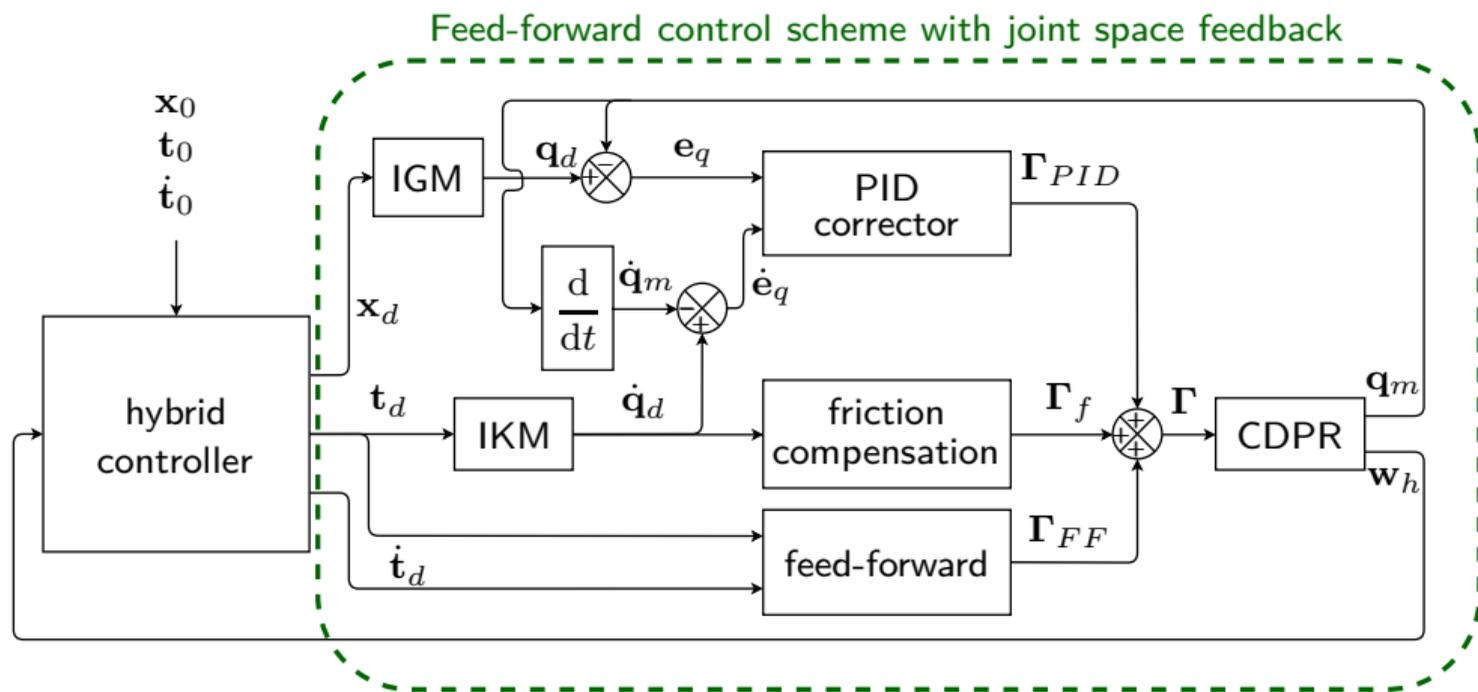
Figure 8: Hybrid control scheme for co-manipulation with a CDPR
