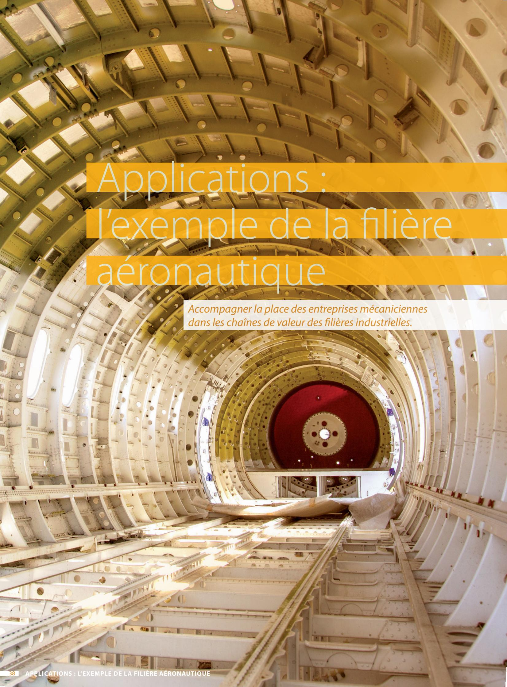
A detailed view of the interior of an aircraft fuselage during construction. The image shows a complex network of white metal ribs and stringers forming a cylindrical structure. At the far end, a large circular opening reveals a red interior. The perspective is from the front of the fuselage looking back towards the tail.
